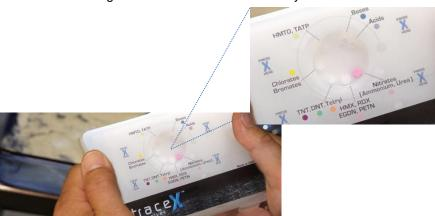
**Figure 2.** Close up view of TraceX showing Nitrates indication.
